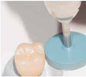
9736H: Trimming the contact points, recommended rotary speed: 10,000 – 15,000 rpm
