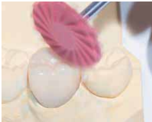
9771F: High shine polishing of the entire crown without high pressure, recommended rotary speed: 10,000 – 15,000 rpm
