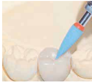
DCA04: Smoothing of the occlusal surface, recommended rotary speed: 10,000 – 15,000 rpm
